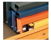
Pallets are placed on nested carts riding on inclined rails.
