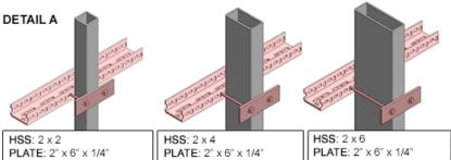
PLATE: 2" x 6" x 1/4" BOLT: Carriage bolt 1/4"ø - 3" long or Treaded rod 5/16"ø - 3" long PIPE: 1/2" STD (0.84"ø OD)
