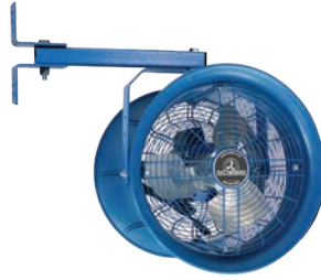
RM: Rack Mount Sizes 14 - 30" 2,600 - 12,000 CFM 50' - 200' Air Throw EC Motor Available Low-profile Mounting
