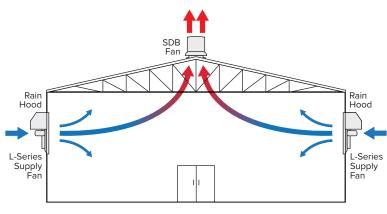
Use roof exhausters in conjunction with supply fans to remove warmer air, fumes, and vapor.
