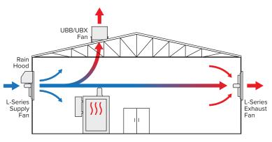
If using a heat producing machine, place a roof exhauster directly above the machine to dispell heat, while also ventilating the whole building through supply and exhaust fans.
