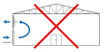
An example of a *poorly* setup system. Air flows in and out of the same area, resulting in no air flow for the rest of the building.
