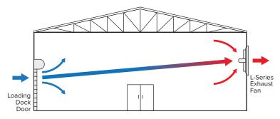
Place exhaust fan on opposite wall of a loading dock door. Only run exhaust when dock door is open.
