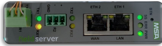
Figure 6 – Gateway power good indication LED
