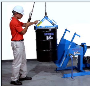
Load upright drum with crane and secure
