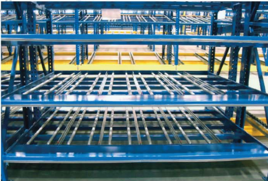
Optional impact deck helps prevent track damage.
