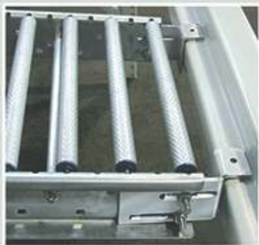
RhinoTrac Brackets Rest on Beam Ledge
