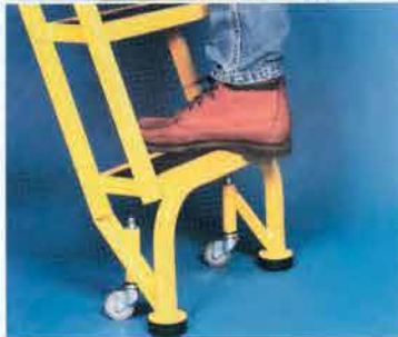
All steps are covered with slip-resistant abrasive matting. Swivel casters at bottom retract while in use and the ladder rests on rubber pad legs.
