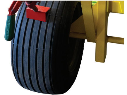
Wide flat free tires exert less pressure on the roof
