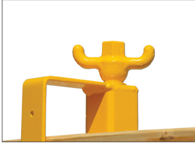
Tighten clamp manually or use a speed wrench.
