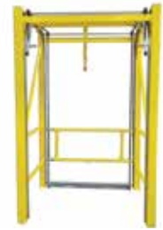
As inboard gate fully opens, leading edge gate is fully closed maintaining fall compliance.
