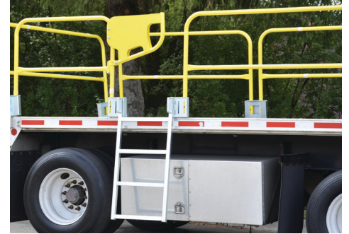
Safety gate protects ladder opening.
