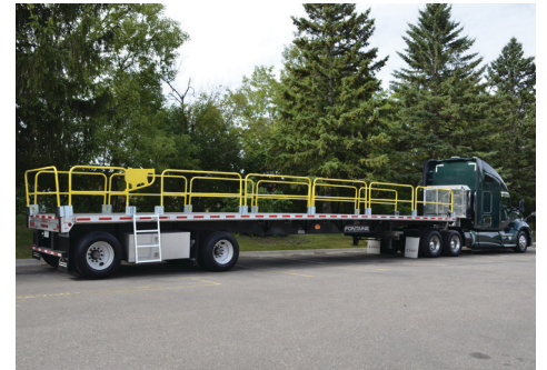
Full protection can be set up in 10 minutes with two workers.
