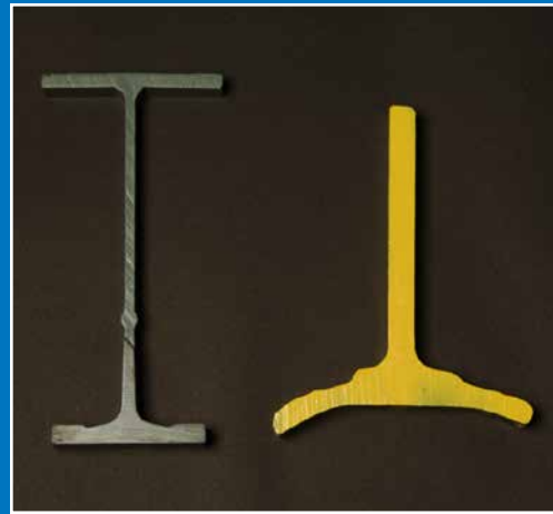
Peening caused the mild steel flange on this I-beam (on right) to bend, making it completely unsafe for crane travel.
