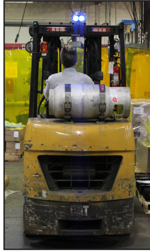
The bright focused beam provides ample warning to pedestrians and other forklifts in the area.
