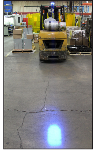
The bright focused beam provides ample warning to pedestrians and other forklifts in the area.
