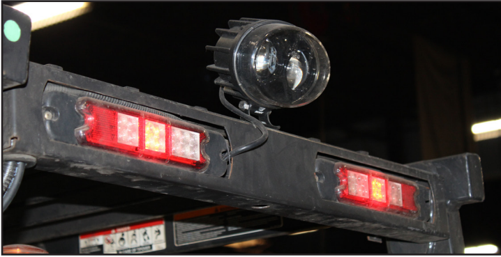
TRUCK-E light shown wired into the lights and mounted on rear portion of the forklift's overhead guard.
