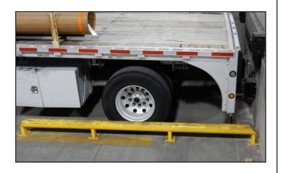
Wheel Guides from Allied Solutions help to ensure trailers enter your loading docks positioned correctly.
