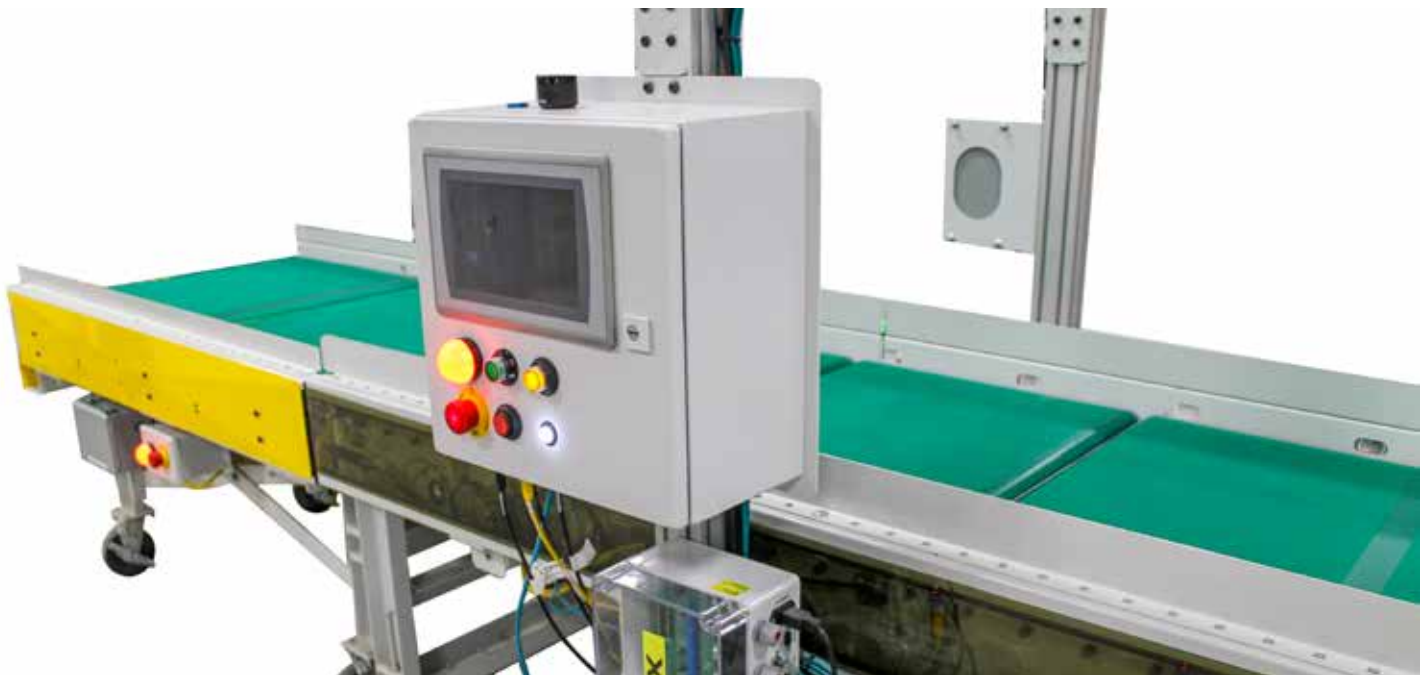
HMI control panel
