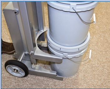
Lifting yoke holds pails in place.
