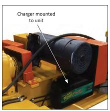
Optional power source for all motorized sheet lifters. Just attached to your crane, no power cord needed! Provides full-time or auxiliary power in case of power failure.
