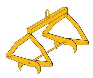
This Dual Gripping Tong system will support and stabilize longer, larger loads that can sustain the force of the entire load on a smaller surface area. When the narrow gripping arms engage the item, significant pressure will be applied. Ideal for handling bundles of steel that are round in shape.
