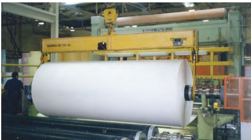
Choose the Model 23 with a fixed-length beam when your roll width doesn't change. J-hook lengths will vary based on roll diameters.
