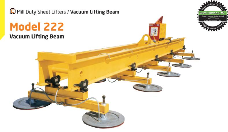
These **Vacuum Lifting Beams** are designed to handle large sheets or plates of metal in the primary metal industry, as well as various other industries. Designed to your material weight and size requirements, units are operated with a pendant, crane-mounted controls, or radio controls. Lifting beams are custom designed per application.
