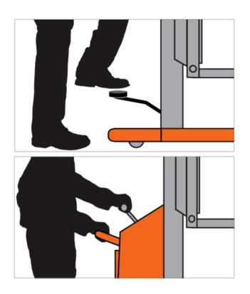
Presto Stackers are available with either manual or powered lift. Manual lift styles include footpump, hand-pump and hand crank. While the amount of work necessary to actuate the lifting mechanism is not unreasonable, manual lifts are best suited for lighter loads and less frequent use. Powered lift stackers are available with AC or DC electric motors to lift loads at the touch of a button. Select a powered lift stacker when dealing with heavier weights or higher duty cycles.
