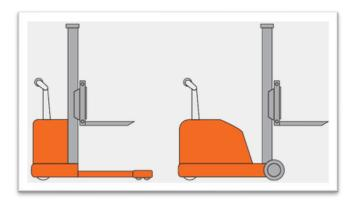
transfer loads from grade to dock level or anywhere that base legs could get in the way, a counterweight stacker should be selected.
