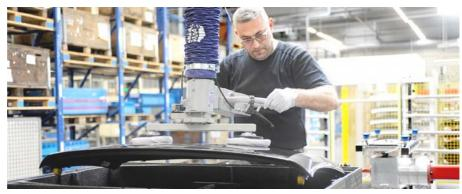
operating elements and grippers and are each designed for specific applications. This makes the vacuum tube lifter not only an ideal helper for machine loading, shipping and order picking areas and many other lifting tasks, it also reduces handling times and thus increases productivity in numerous industries.
