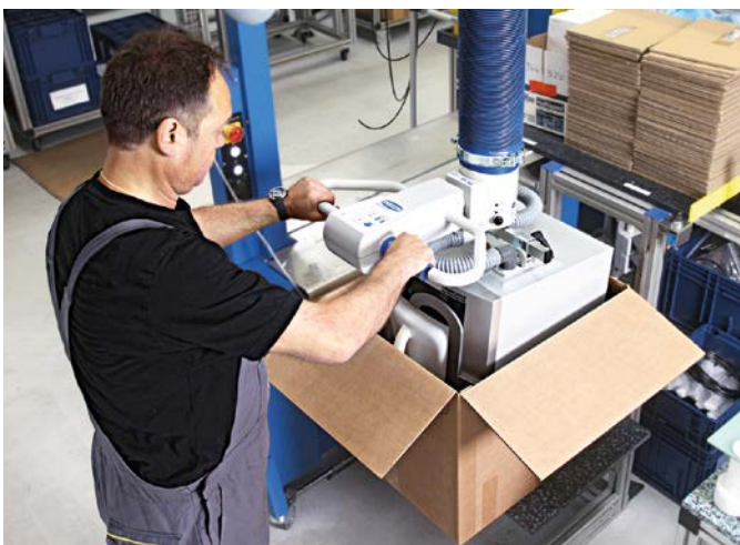
Vacuum tube lifter JumboErgo for packaging goods into boxes and handling the sealed boxes
