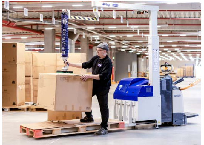
Vacuum tube lifter JumboFlex Picker for mobile picking of packages with any common industrial truck
