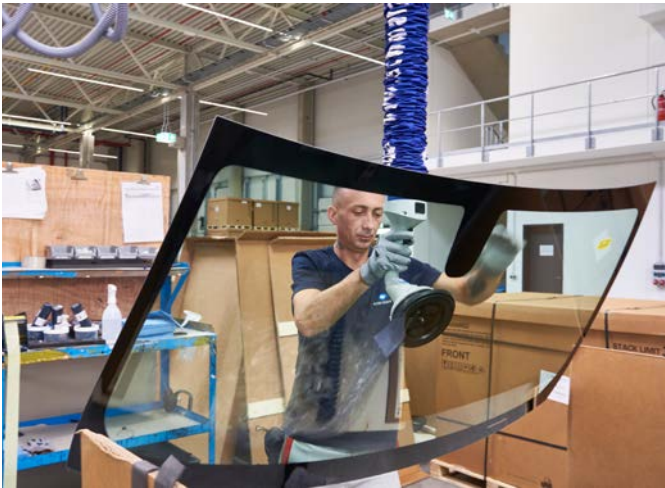
Vacuum tube lifter JumboFlex for handling windshields
