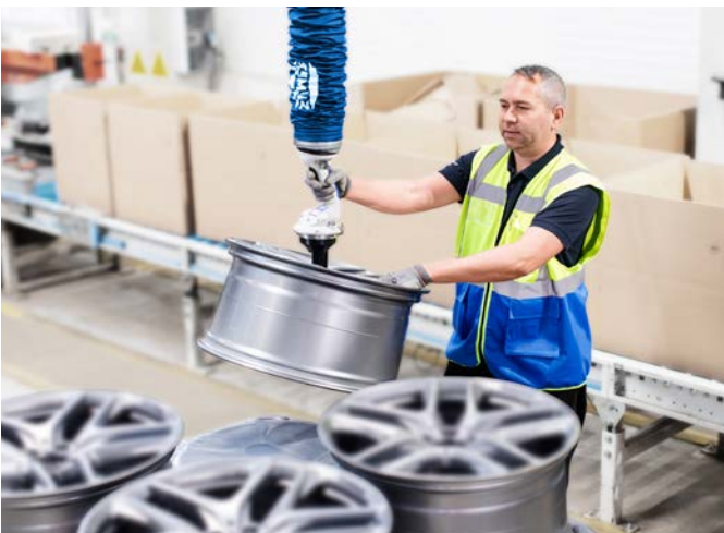
Vacuum tube lifter JumboFlex with rim gripper for handling rims and complete wheels
