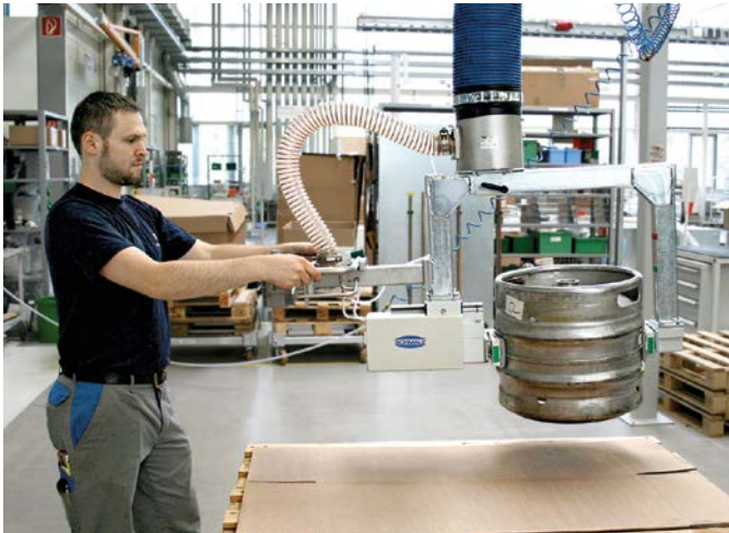
Beverages | Vacuum tube lifter JumboErgo with mechanical grippers for lifting and turning kegs
