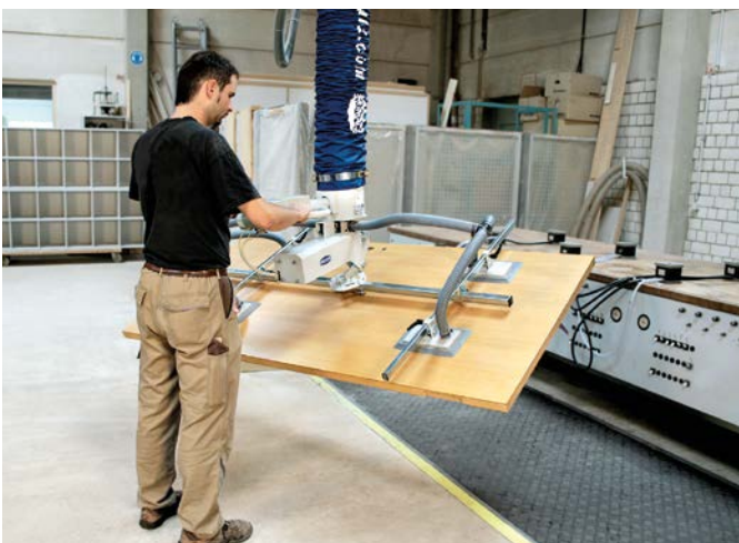
Vacuum tube lifter JumboErgo with 90° swivel angle for loading a CNC machining center
