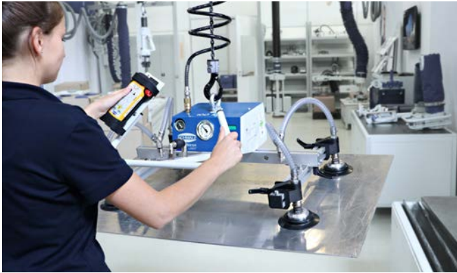
VacuMaster Light for handling metal sheets
