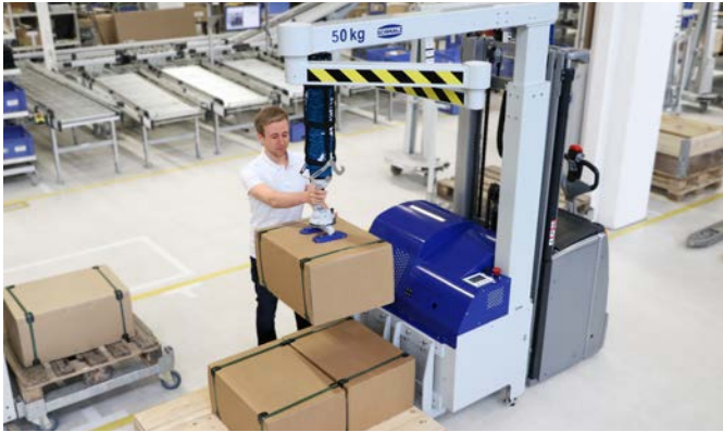
JumboFlex Picker for mobile use in order picking tasks
