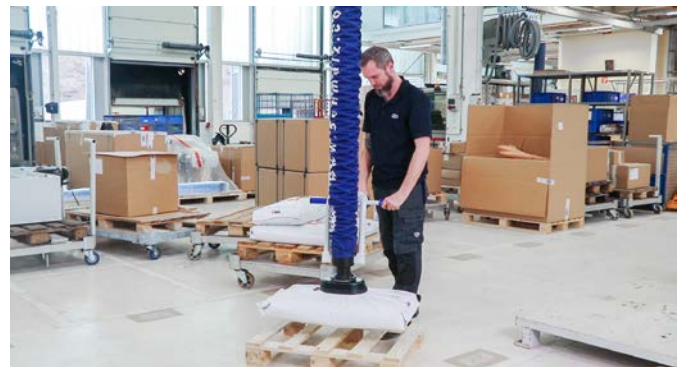
JumboFlex High-Stack when handling bags
