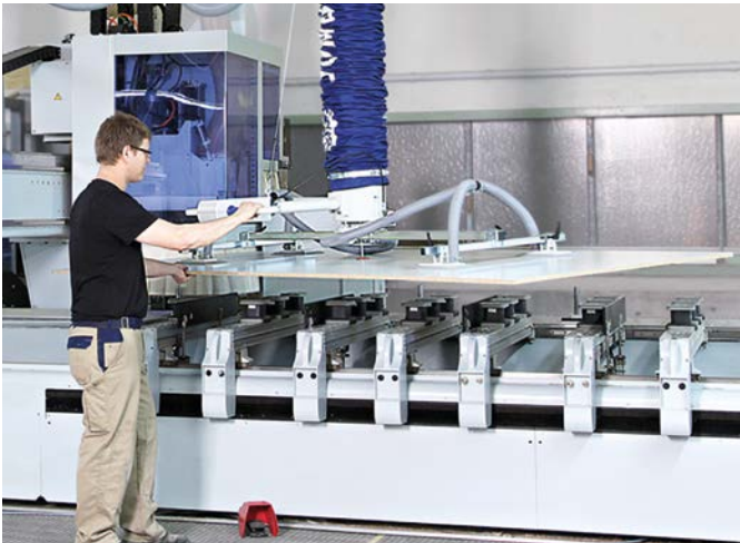
Vacuum tube lifter JumboErgo for loading and unloading a CNC machining center
