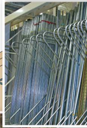
Separate pipe or tubing stored vertically
