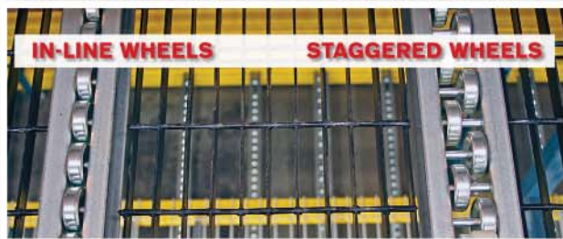
Staggered Wheels for heavier loads - 1 1/2" - 2" centers
