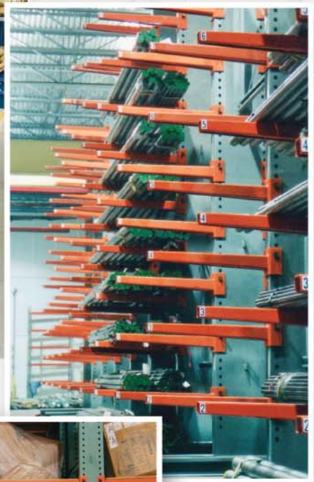
Pipe storage cantilever
