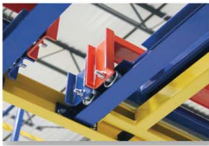
Carts flow automatically on four sealed wheels
