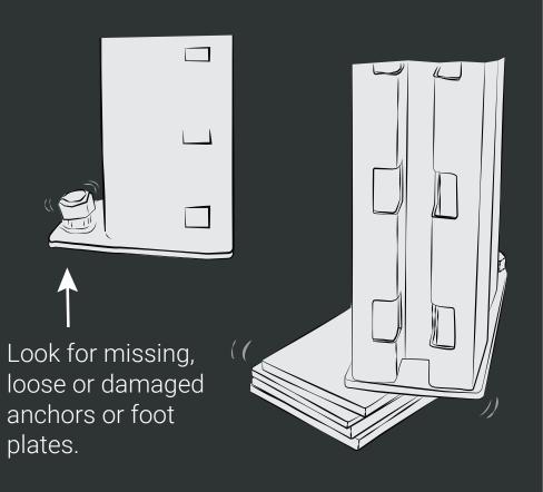
Shims should be well seated, secured and of equal size to the footplate.
