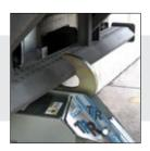
The TPR hook rotates up to engage the even the toughest pentagonal shaped RIG and secure the trailer to the loading dock.
