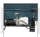
Convenient under dock mount of motor/ pump with translucent reservoir for ease of maintenance.
